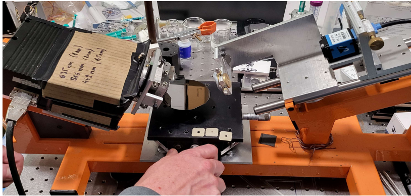
Figure 35. RGB laser, pinhole-polarizer-(optional) compensator, sample, sample-holder, polarization-sensitive camera.
