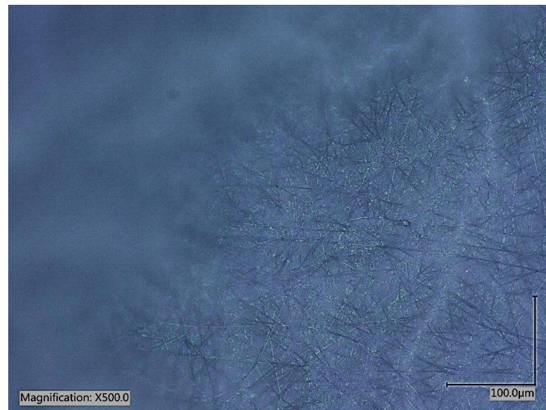
Microscopic examination of CA polymer fiber of different concentrations (5, 10, 15, 16, 18, 20) % in acetone–DMF (2:1)
