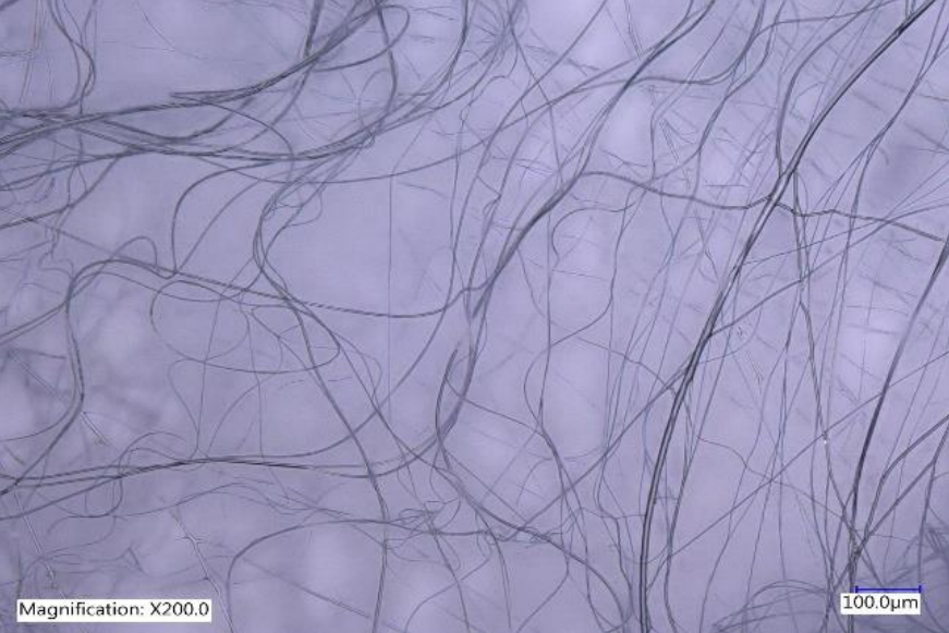
Microscopic examination of generated fiber of PVP polymer with different magnification
