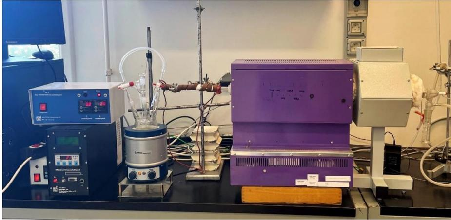
High temperature oxidation furnace in air and steam
