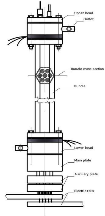
**Test section with seven-rod bundle**
