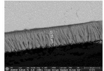
Thickness of the Cr layer on spacer grid :
