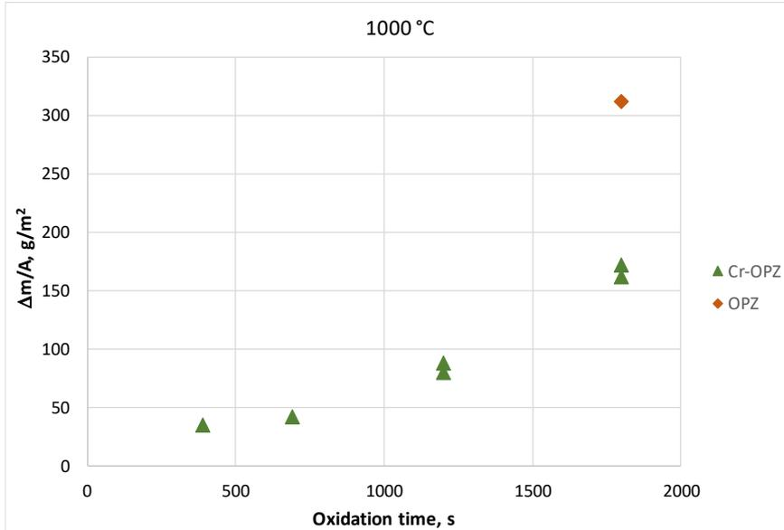
Mass gain of uncoated and coated optZIRLO alloy
