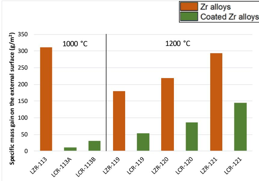
Comparing of Specific mass gain at isothermal Temperature :
