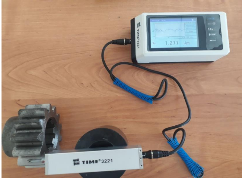
Measurement of surface roughness in grinding process using TIME 3221 digital profilometer (A typical portable instrument)
