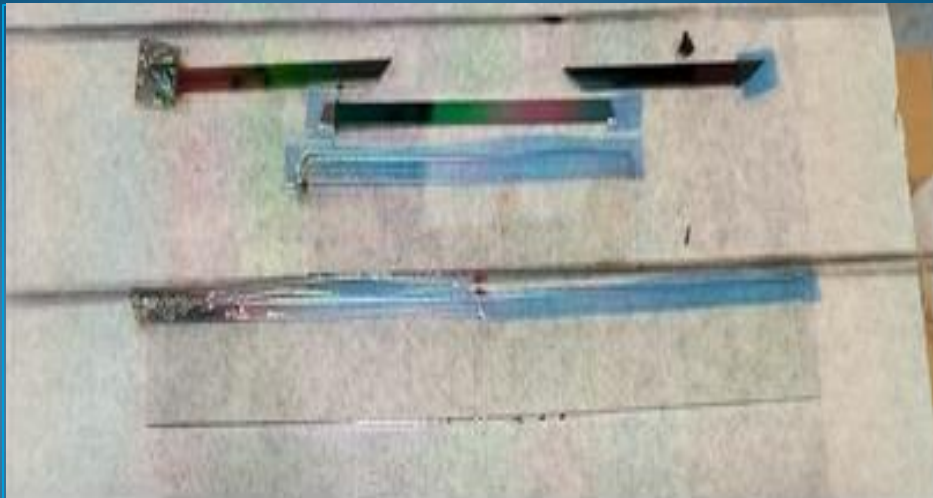
Figure (2) \text{TiO}_2\text{-MoO}_3 , ITO- covered glass and Si-probes on a glass substrate, before-electrochromic-experiments, the Ti-rich in the left side and the Mo-rich in the right side .
