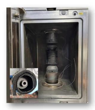
SPS settings for high entropy ceramics (HECs) involve controlling key parameters such as temperature gradient, current density, material conductivity, mold wall thickness, current pattern, heating rate, holding time, and sintering pressure. These parameters vary depending on the desired properties for each experiment.
