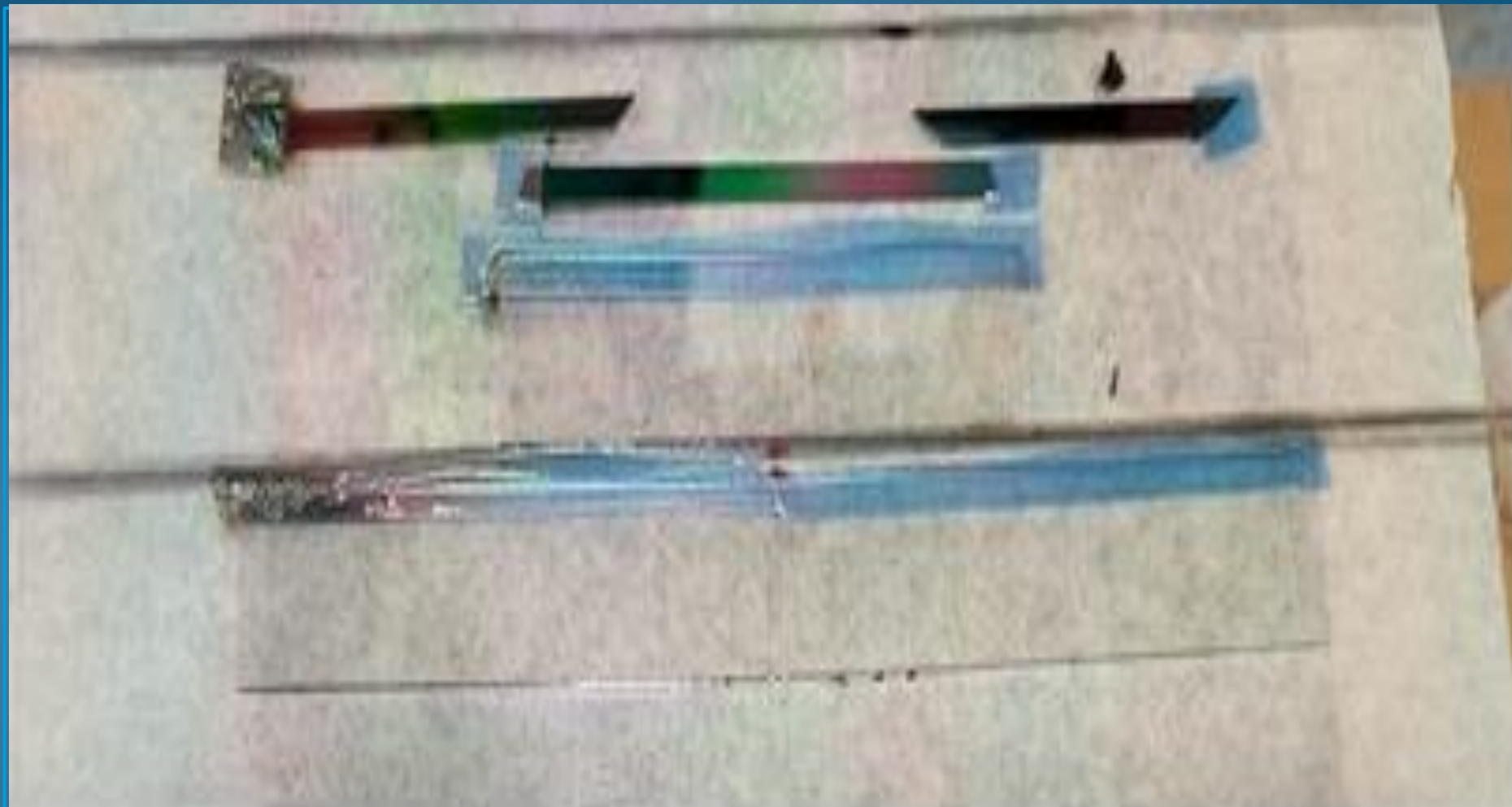
Figure (3) \text{TiO}_2\text{-MoO}_3 , ITO- covered glass and Si-probes on a glass substrate, before-electrochromic-experiments, the Ti-rich in the left side and the Mo-rich in the right side .
