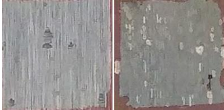
Figure 16. N. 1. samples: a) without heat treatment, b) heat treated
