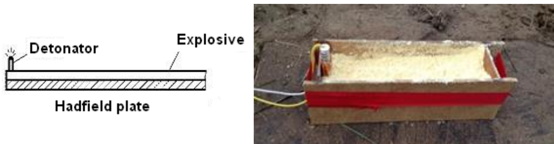
Figure 7. Setup of the direct explosion hardening [22]
