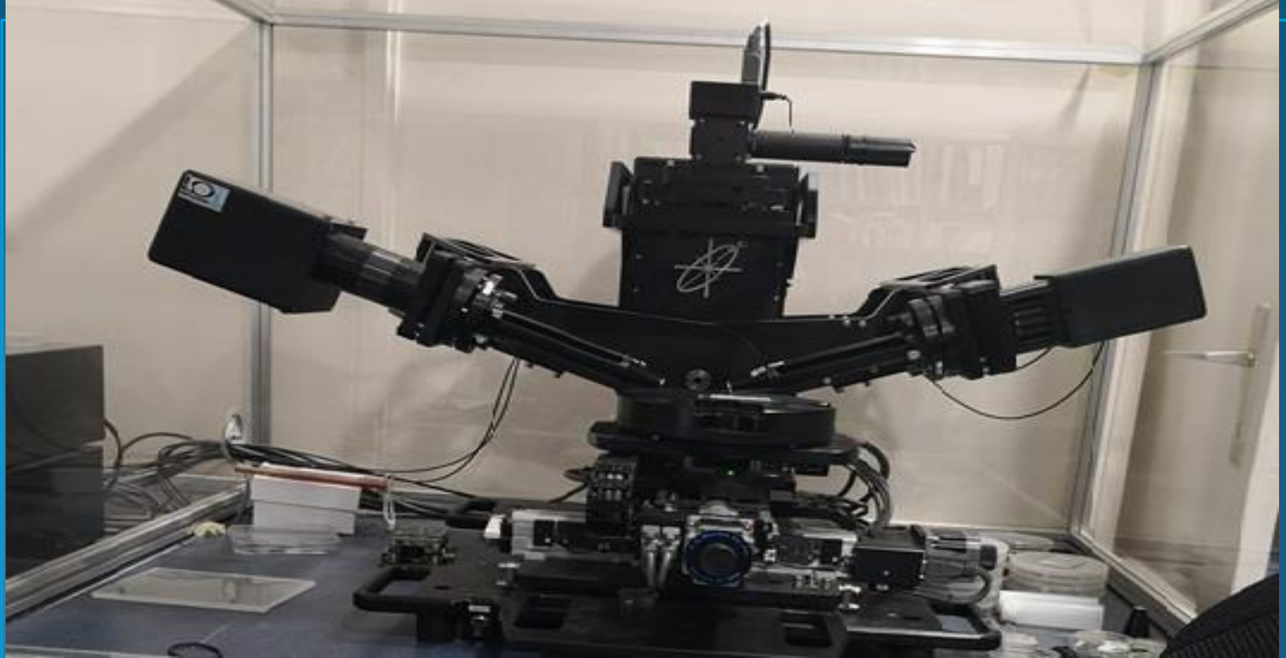
Figure (3) a) Spectroscopic Ellipsometry device, Woollam M-2000DI, Wavelength range from 191-1690 nm (photon energies from 0.7-6.5 eV), Automatic scan with a micro-focused 0.2 mm spot. Angle of incidence: 45-75 degree. Measurement time 1 sec per spot.
