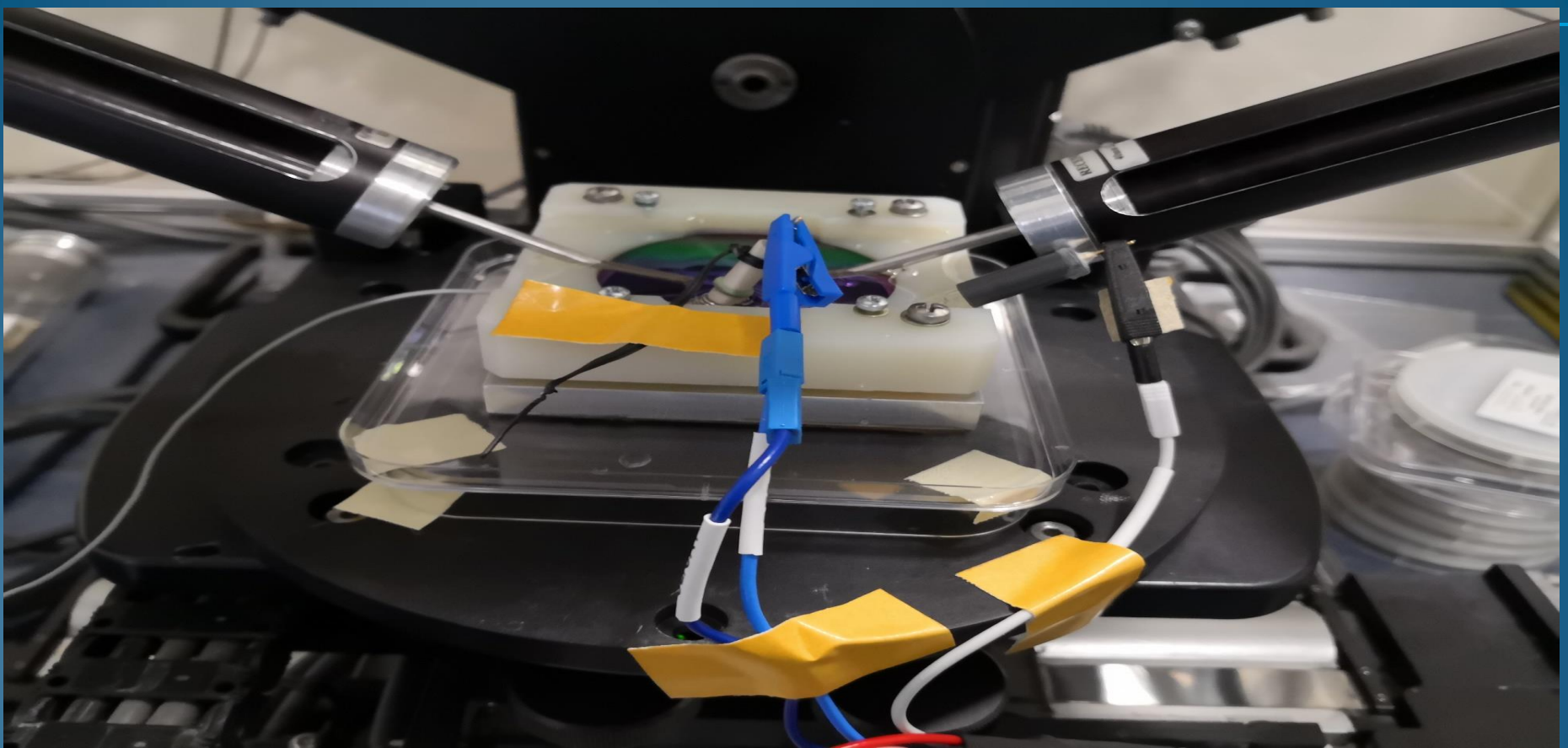
Figure (15) Electrochemical measurements were performed in a circular cell filled with 1M lithium perchlorate ( \text{LiClO}_4 ) / propylene carbonate electrolyte, and a Pt wire counter electrode was placed into the electrolyte alongside with a reference electrode.
