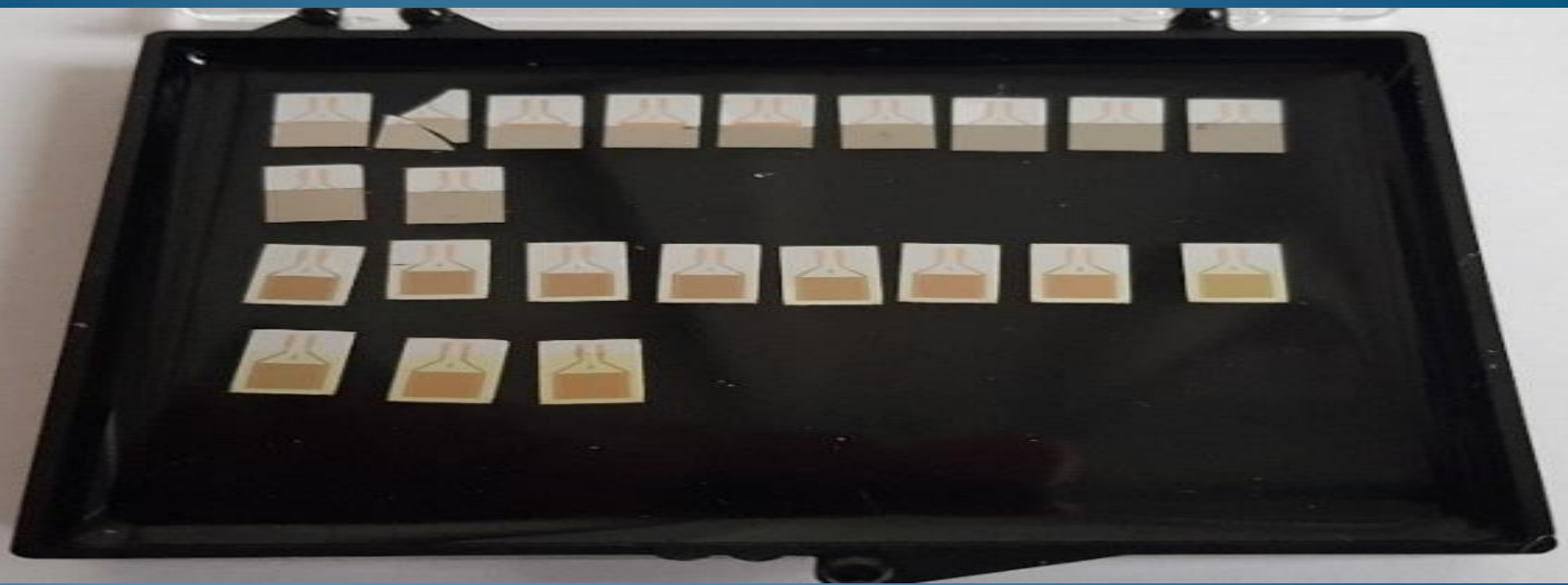
Fig. 10 Photographs (from different view-angle) of \text{WO}_3/\text{MoO}_3 (lower) or \text{WO}_{3-x}/\text{MoO}_{3-x} (upper) combinatorial sets on heat-able sensor chips. Left hand side is W-rich, right one is Mo-rich. No. 6 (middle one) is expected to be 50-50% in both cases. The upper rows show sub oxides (semi-transparent layers, No. 2 was broken during tweezer handling) The bottom rows show oxides (transparent layers).
