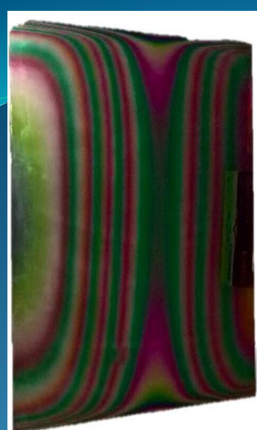
Figure (1) Schematic picture of the deposition arrangement and the photograph of 30x30 cm substrate with composition-gradient layers. Colored bands show thickness and composition gradient.
