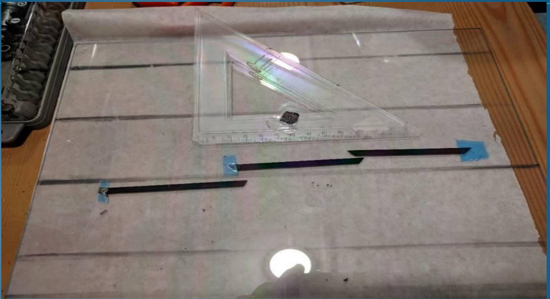
Fig. 12 Ti and Sn oxides combinatorial deposition. Silicon probes to measure the thickness and composition map.
