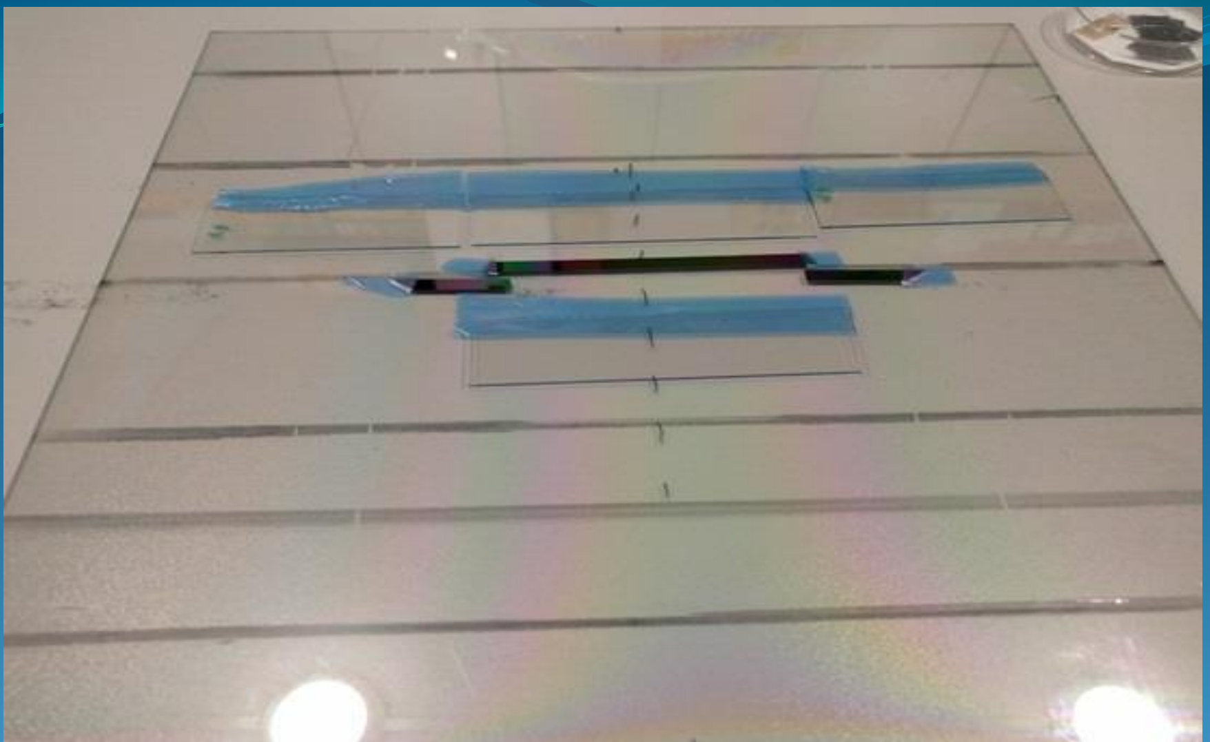
Figure (5) WO 3 -MoO 3 combinatorial mixed layers on glass- and Si-substrates on top of a 30x30 cm glass sheet. The pale colored bands show the changing thicknesses and compositions.
