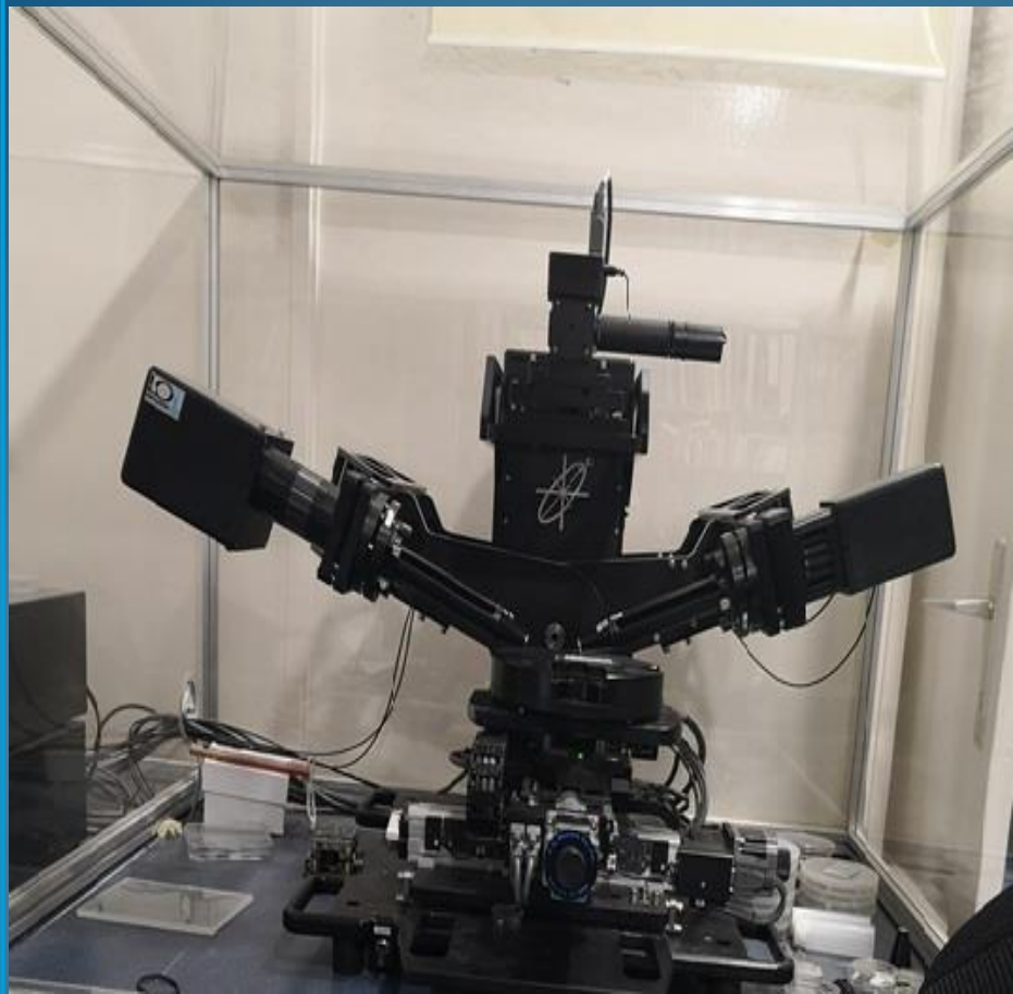
Figure (3) Spectroscopic Ellipsometry devices, a) Woollam M-2000DI, b) imaging ellipsometer (Source: http://www.ellipsometry.hu/#Equipment ) and the data analysis parameters for the device.
