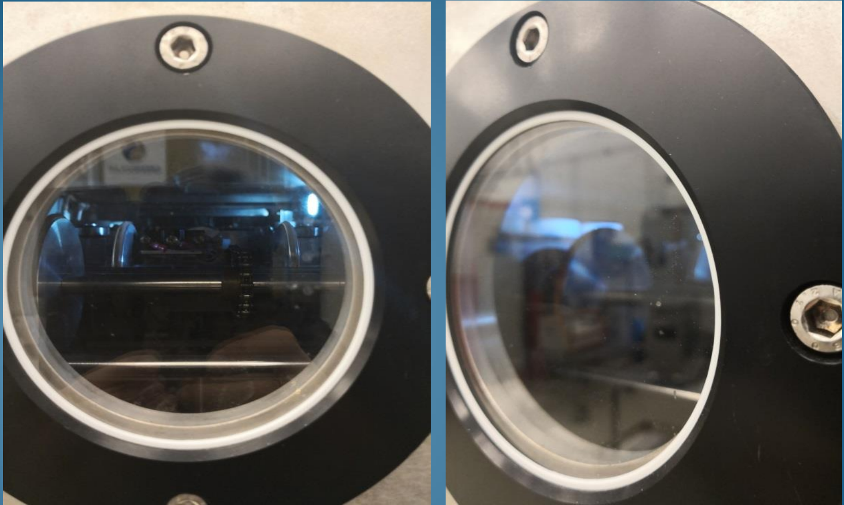
Figure (2) the chamber for DC magnetron sputtering device after air vacuumed. Blue light is from the Ar-O 2 plasma.
