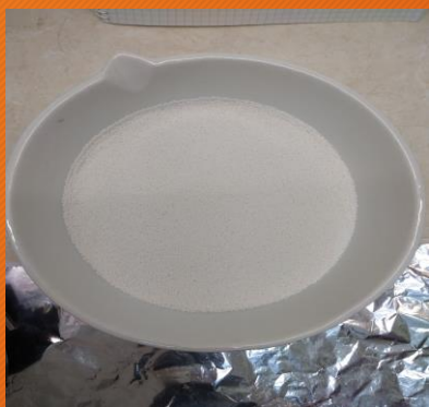
Zirconia balls, 1mm in diameter
