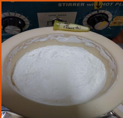
Milled Silica gel after 3 hours (Silica powder)
