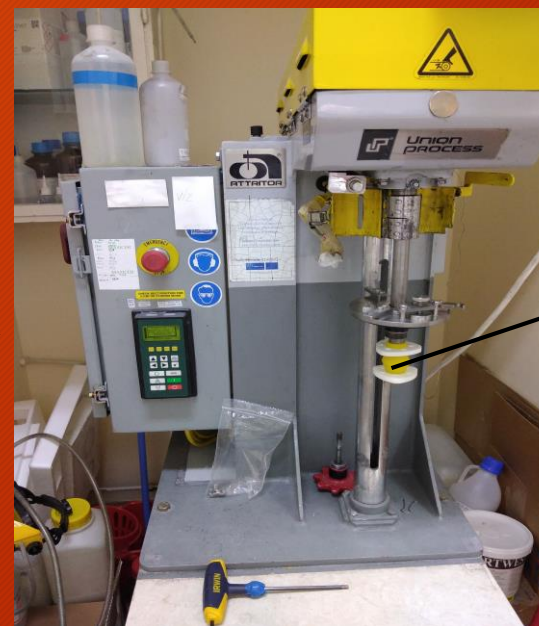
Attrition milling in wet conditions at 2000 rpm for 3h
