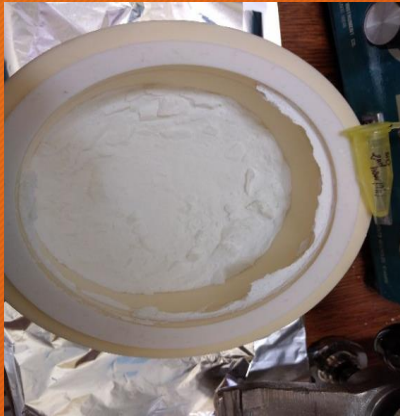
Milled Silica gel after 2 hours
