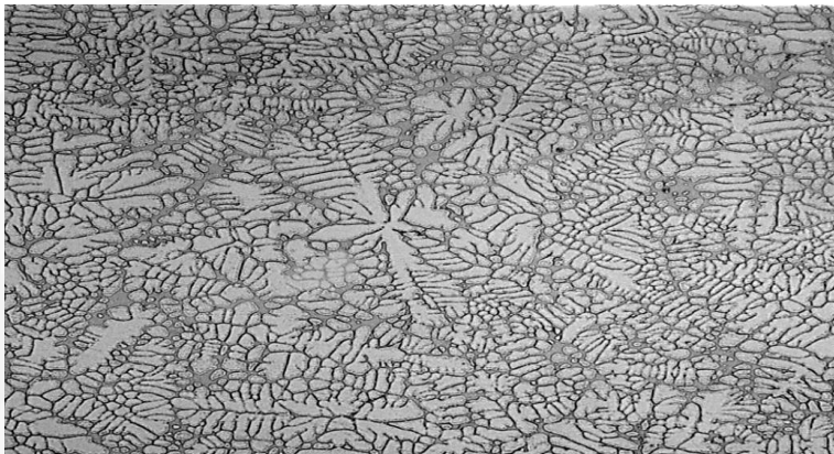
Figure 3. a. Typical Dendritic Microstructure
