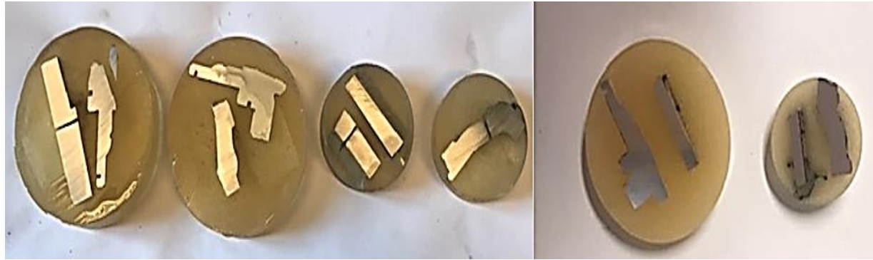
Figure 19 Casting and Rheocasting application mounting samples
