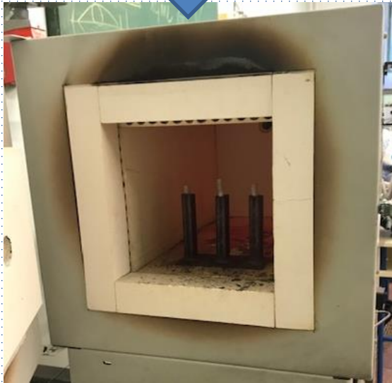
Figure 13. Rheocasting process active in the present work: (a) solid block of the same alloy prepared in advance, attached to a stainless steel rod, (b) dissolved in the melt with simultaneous stirring action, and (c) the slurry thus produced.
