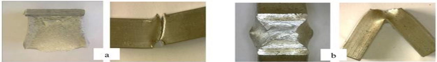
Figure (13) a. Front and side view of as-cast Specimen in 0°C, b. Front and side view of the casting Specimen in 0°C
