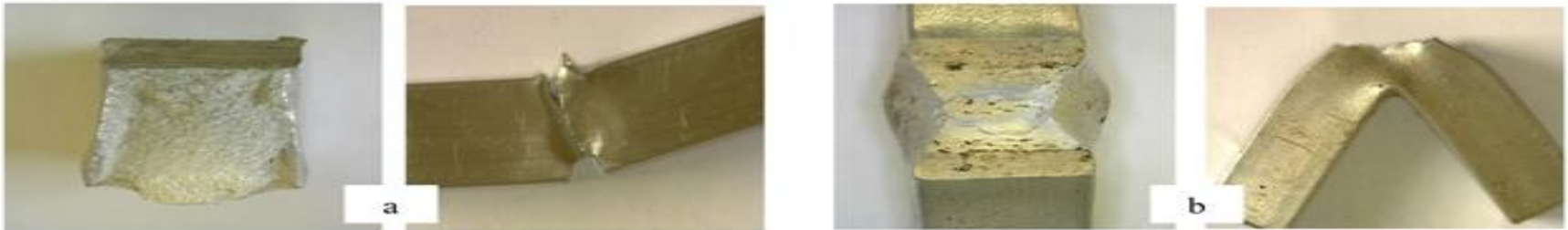
Figure (16) a. Front and side view of as-cast Specimen in 100 °C, b. Front and side view of rheocasting Specimen in 100°C
