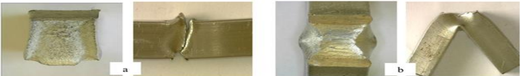
Figure (15) a. Front and side view of as-cast Specimen in 40 °C, b. Front and side view of theocasting Specimen in 40°C
