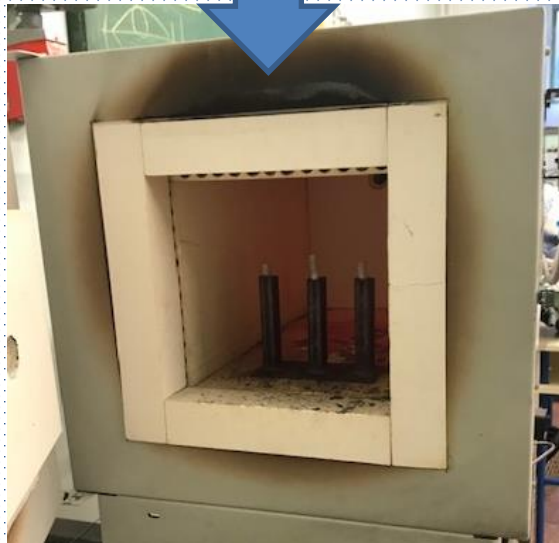
Figure 10. Rheocasting process active in the present work: (a) solid block of the same alloy prepared in advance, attached to a stainless steel rod, (b) dissolved in the melt with simultaneous stirring action, and (c) the slurry thus produced.
