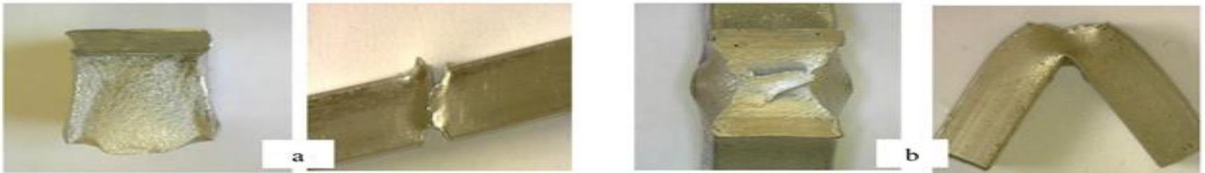
Figure (17) a. Front and side view of as-cast Specimen in -25 °C, b. Front and side view of rheocasting Specimen in -25°C
