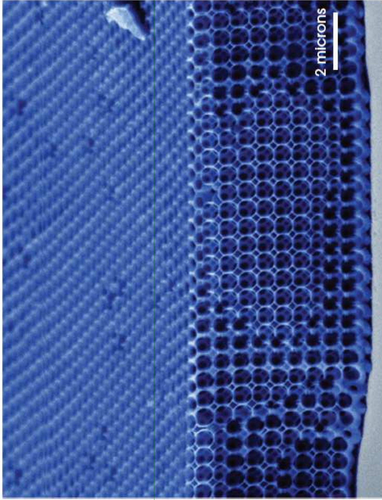
Figure 9: Electron-microscope image (artificial coloring) of inverse-opal structure demonstrated to have a complete band gap around a wavelength of 1.3 microns in Vlasov et al. (2001). Unlike figure 8, this is actually an fcc lattice of hollow dielectric (silicon) shells, which increases the size of the gap. (Image courtesy D. J. Norris.)
