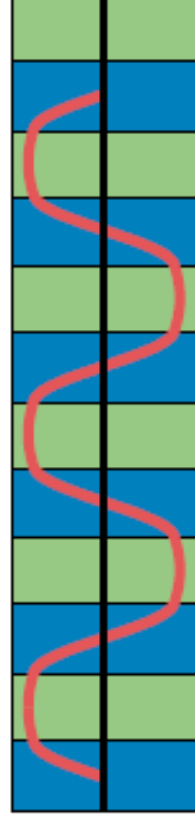
(b) E-field for mode at bottom of band 2
