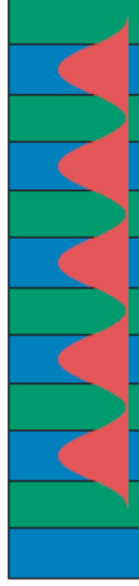
(c) Local energy density in E-field, top of band 1
