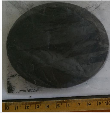
0,33 wt% Si 3 N 4 Sintered at 900 C° for 5 min
