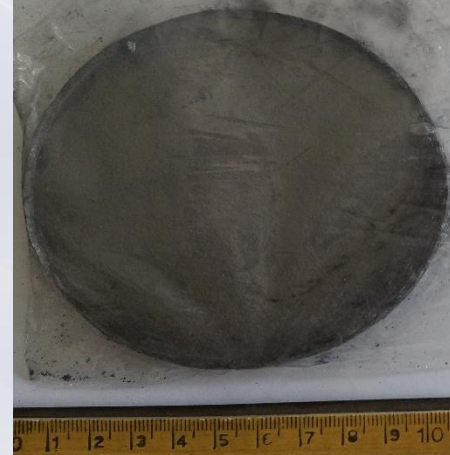
1 wt% SiC Sintered at 900 C° for 5 min
