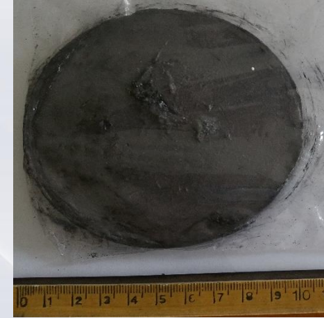
0,33 wt% Y 2 O 3 Sintered at 900 C° for 5 min
