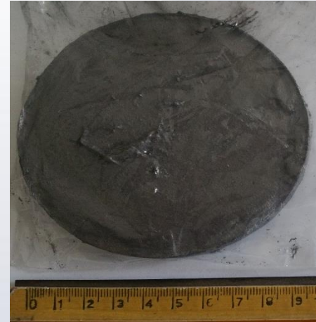
1wt% Y 2 O 3 Sintered at 900 C° for 5 min
