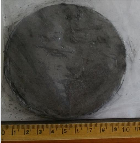
1wt% Si 3 N 4 Sintered at 900 C° for 5 min
