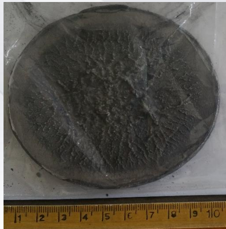
0,33 wt% SiC Sintered at 950 C° for 10 min
