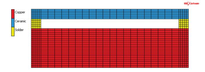
Using the results from the Anand Model, power-law parameters were obtained for SAC305 solder. The accuracy of the results is acceptable with an error of nearly 10% as compared to the simulation values. However, the method used was based on the principle of relative error.
