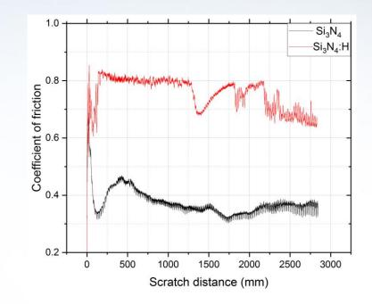
Refractive index and extinction coefficient are decreased while hydrogen flow is increased Presence of hydrogen increases the coefficient of friction of the thin film
