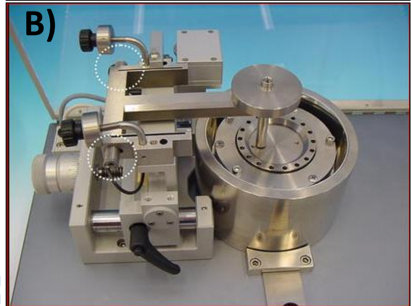
Fig.1 A) schematic design and B) real instrument of High temperature Tribometer.
