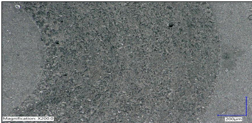
Fig.2 Wear track in the composite with 5 wt. % /MWCNTs recorded by Kenyence Microscopy
